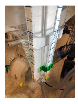
Level sensor on front, because of the 90 angles the sensor is difficult to maintain metal contact.
